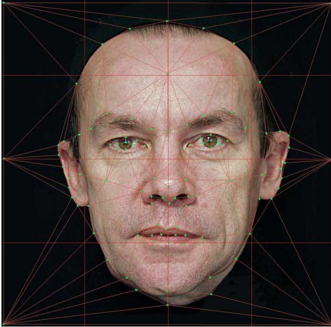
Figure 1. Example of the meshes used for implementing the morphing algorithm. Two sets of points are used to identify the corresponding features of the two faces. Each set of points is connected by a Delaunay triangulation, which is known to provide the optimal solution to the problem of interpolating a two-dimensional landscape f(x,y) to a finite set of samples. Because Delaunay triangulations are uniquely defined, the tessellations of the two images are topologically identical. [Colour versions of all figures are available online].
